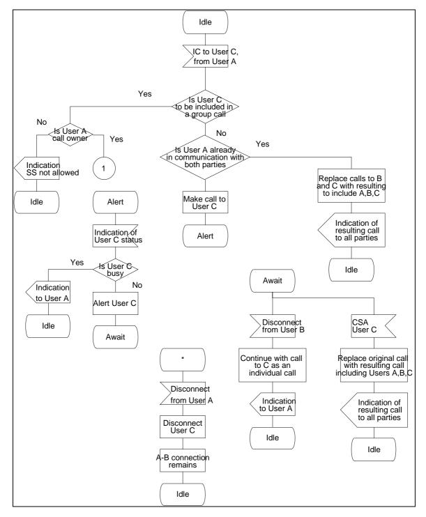
Figure 1: Sheet 1 of 2, SS IC, overall SDL
